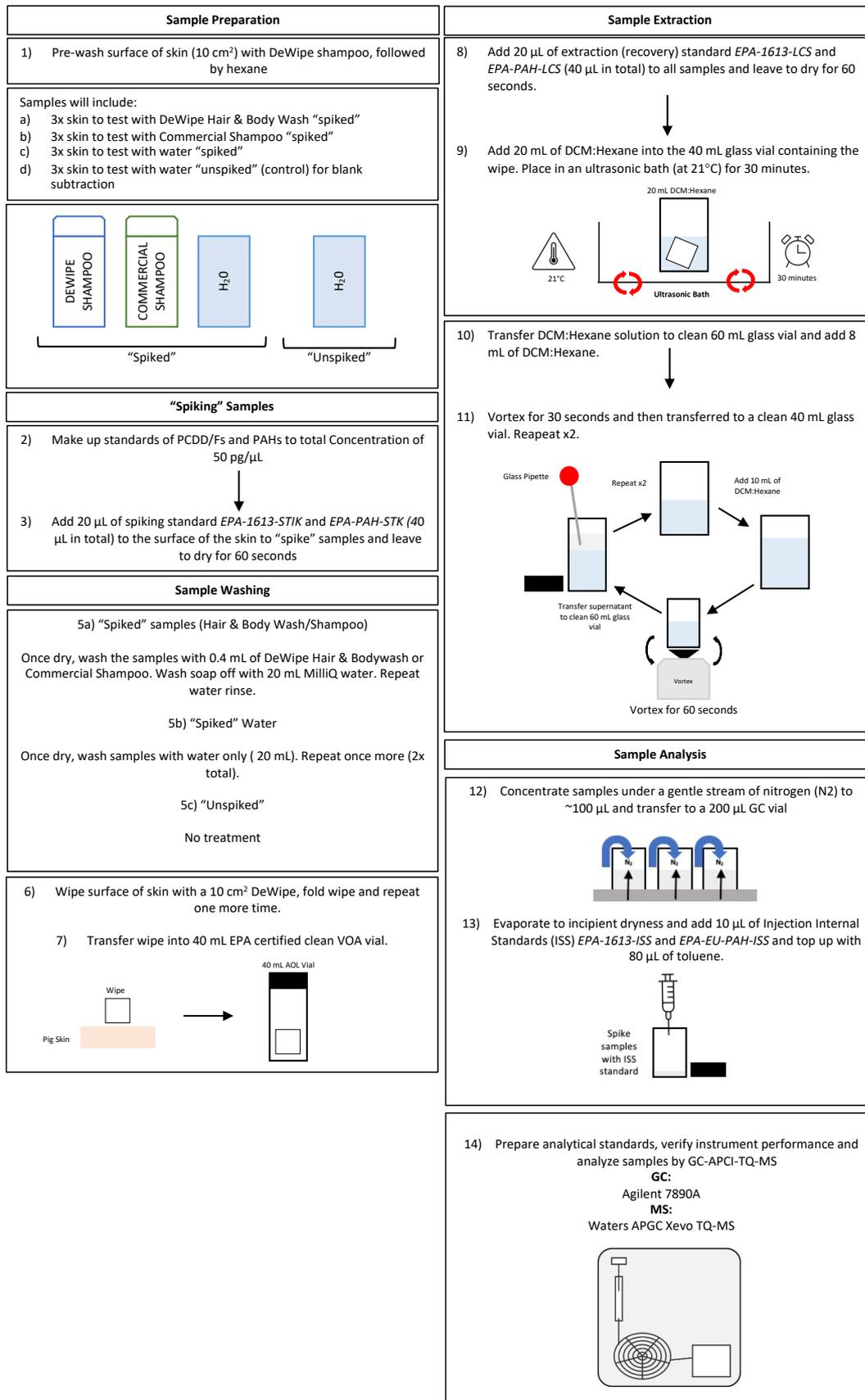
Figure 1. Schematic overview of extraction method for dioxins, furans and PAHs from skin, wiped with a De-Wipe.
